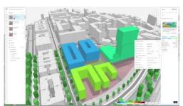
Powered by machine learning, Forma's rapid operational energy analysis allows architects to easily assess the impact of design decisions on the potential operational energy of their buildings during early-phase design. Image Courtesy of Autodesk
